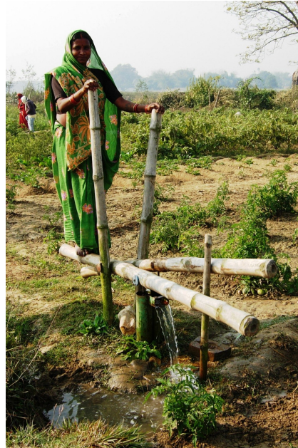
Figure 1: Bamboo treadle pumps are used for irrigation in Nepal. Photo: Practical Action / Sandra Gibson.
